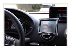
In the words of Víctor Iglesias, Ficosa's Systems Architect: "The electronic mirror offers a new safer and more comfortable driving experience through the inclusion in the vision systems of ADAS (Advanced Systems Driver Assistance), as the traffic detection function, which provides information to the driver about the vehicles around it".
