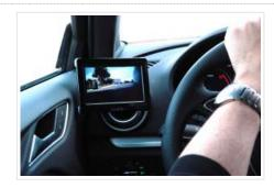
Ficosa has developed an electronic mirror composed of cameras and displays which implies an alternative option to the exterior rear-view mirrors of the car. This pioneering system, also known as CMS (Camera Monitor System), represents an authentic revolution for the automotive industry as well as an important progress towards the autonomous car.
