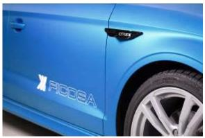
The electronic mirror stands out for expanding the field of view, eliminating blind spots. In turn, the small size of the cameras greatly improves the car aerodynamic coefficient which involves a reduction of fuel consumption and the wind noise perceived from inside the vehicle.
